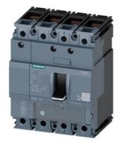
circuit breaker 3VA1 IEC frame 160 breaking capacity class S Icu=36kA @ 415V 4-pole, line protection TM220, ATFM, In=63A overload protection Ir=44A...63A short-circuit protection Ii=10 x In N conductor unprotected nut keeper kit
