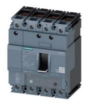
circuit breaker 3VA1 IEC frame 160 breaking capacity class N Icu=25kA @ 415V 4-pole, line protection TM240, ATAM, In=63A overload protection Ir=44A...63A short-circuit protection Ii=5...10 x In N conductor protection 100% clamp connection
