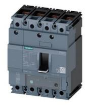
circuit breaker 3VA1 IEC frame 160 breaking capacity class N Icu=25kA @ 415V 4-pole, line protection TM240, ATAM, In=63A overload protection Ir=44A...63A short-circuit protection Ii=5...10 x In N conductor protection 100% nut keeper kit
