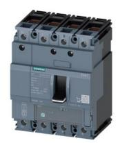
circuit breaker 3VA1 IEC frame 160 breaking capacity class N lcu=25kA @ 415V 4-pole, line protection TM220, ATFM, In=63A overload protection Ir=44A...63A short-circuit protection li=10 x In N conductor protection 100% clamp connection
