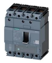
circuit breaker 3VA1 IEC frame 160 breaking capacity class N Icu=25kA @ 415V 4-pole, line protection TM220, ATFM, In=63A overload protection Ir=44A...63A short-circuit protection Ii=10 x In N conductor protection 100% nut keeper kit
