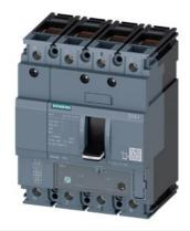
circuit breaker 3VA1 IEC frame 160 breaking capacity class N Icu=25kA @ 415V 4-pole, line protection TM240, ATAM, In=63A overload protection Ir=44A...63A short-circuit protection Ii=5...10 x In N conductor unprotected clamp connection
