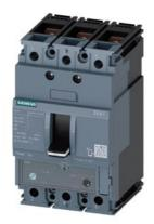
circuit breaker 3VA1 IEC frame 160 breaking capacity class N Icu=25kA @ 415V 3-pole, line protection TM240, ATAM, In=63A overload protection Ir=44A...63A short-circuit protection Ii=5...10 x In nut keeper kit
