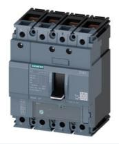
circuit breaker 3VA1 IEC frame 160 breaking capacity class N Icu=25kA @ 415V 4-pole, line protection TM220, ATFM, In=63A overload protection Ir=44A...63A short-circuit protection Ii=10 x In N conductor unprotected nut keeper kit
