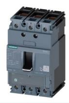
circuit breaker 3VA1 IEC frame 160 breaking capacity class N Icu=25kA @ 415V 3-pole, line protection TM220, ATFM, In=63A overload protection Ir=44A...63A short-circuit protection Ii=10 x In clamp connection
