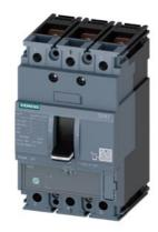
circuit breaker 3VA1 IEC frame 160 breaking capacity class N Icu=25kA @ 415V 3-pole, line protection TM220, ATFM, In=63A overload protection Ir=44A...63A short-circuit protection Ii=10 x In nut keeper kit
