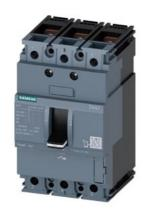
circuit breaker 3VA1 IEC frame 160 breaking capacity class N Icu=25kA @ 415V 3-pole, line protection TM210, FTFM, In=63A overload protection Ir=63A fixed short-circuit protection Ii=10 x In nut keeper kit
