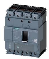
circuit breaker 3VA1 IEC frame 160 breaking capacity class M Icu=55kA @ 415V 4-pole, line protection TM220, ATFM, In=50A overload protection Ir=35A...50A short-circuit protection Ii=10 x In N conductor protection 100% clamp connection
