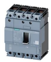
circuit breaker 3VA1 IEC frame 160 breaking capacity class M Icu=55kA @ 415V 4-pole, line protection TM210, FTFM, In=50A overload protection Ir=50A fixed short-circuit protection Ii=10 x In N conductor protection 100% nut keeper kit
