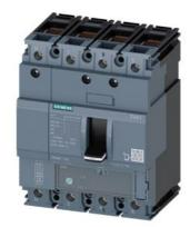
circuit breaker 3VA1 IEC frame 160 breaking capacity class M Icu=55kA @ 415V 4-pole, line protection TM220, ATFM, In=50A overload protection Ir=35A...50A short-circuit protection Ii=10 x In N conductor unprotected clamp connection
