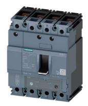
circuit breaker 3VA1 IEC frame 160 breaking capacity class S Icu=36kA @ 415V 4-pole, line protection TM240, ATAM, In=50A overload protection Ir=35A...50A short-circuit protection Ii=5...10 x In N conductor unprotected nut keeper kit
