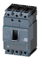
circuit breaker 3VA1 IEC frame 160 breaking capacity class S Icu=36kA @ 415V 3-pole, line protection TM220, ATFM, In=50A overload protection Ir=35A...50A short-circuit protection Ii=10 x In nut keeper kit
