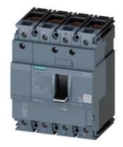
circuit breaker 3VA1 IEC frame 160 breaking capacity class S Icu=36kA @ 415V 4-pole, line protection TM210, FTFM, In=50A overload protection Ir=50A fixed short-circuit protection Ii=10 x In N conductor unprotected clamp connection
