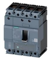
circuit breaker 3VA1 IEC frame 160 breaking capacity class N Icu=25kA @ 415V 4-pole, line protection TM220, ATFM, In=50A overload protection Ir=35A...50A short-circuit protection Ii=10 x In N conductor protection 100% nut keeper kit
