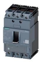
circuit breaker 3VA1 IEC frame 160 breaking capacity class N Icu=25kA @ 415V 3-pole, line protection TM220, ATFM, In=50A overload protection Ir=35A...50A short-circuit protection Ii=10 x In clamp connection
