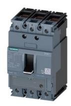
circuit breaker 3VA1 IEC frame 160 breaking capacity class M Icu=55kA @ 415V 3-pole, starter protection TM120M, AM, In=40A without overload protection short-circuit protection Ii=7...16 x In clamp connection
