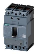
circuit breaker 3VA1 IEC frame 160 breaking capacity class M Icu=55kA @ 415V 3-pole, starter protection TM120M, AM, In=40A without overload protection short-circuit protection li=7...16 x In nut keeper kit
