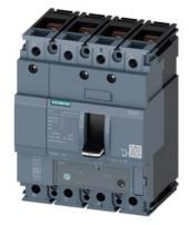
circuit breaker 3VA1 IEC frame 160 breaking capacity class M Icu=55kA @ 415V 4-pole, line protection TM240, ATAM, In=40A overload protection Ir=28A...40A short-circuit protection Ii=5...10 x In N conductor protection 100% nut keeper kit
