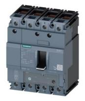
circuit breaker 3VA1 IEC frame 160 breaking capacity class S Icu=36kA @ 415V 4-pole, line protection TM240, ATAM, In=40A overload protection Ir=28A...40A short-circuit protection Ii=5...10 x In N conductor protection 100% clamp connection
