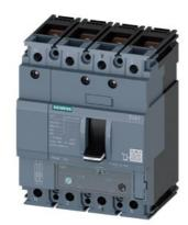
circuit breaker 3VA1 IEC frame 160 breaking capacity class S Icu=36kA @ 415V 4-pole, line protection TM240, ATAM, In=40A overload protection Ir=28A...40A short-circuit protection Ii=5...10 x In N conductor protection 100% nut keeper kit
