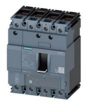
circuit breaker 3VA1 IEC frame 160 breaking capacity class S Icu=36kA @ 415V 4-pole, line protection TM220, ATFM, In=40A overload protection Ir=28A...40A short-circuit protection Ii=10 x In N conductor protection 100% clamp connection
