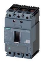
circuit breaker 3VA1 IEC frame 160 breaking capacity class S Icu=36kA @ 415V 3-pole, line protection TM220, ATFM, In=40A overload protection Ir=28A...40A short-circuit protection Ii=10 x In nut keeper kit
