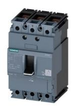
circuit breaker 3VA1 IEC frame 160 breaking capacity class S Icu=36kA @ 415V 3-pole, line protection TM210, FTFM, In=40A overload protection Ir=40A fixed short-circuit protection Ii=10 x In nut keeper kit
