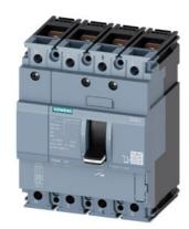
circuit breaker 3VA1 IEC frame 160 breaking capacity class N Icu=25kA @ 415V 4-pole, line protection TM210, FTFM, In=40A overload protection Ir=40A fixed short-circuit protection Ii=10 x In N conductor protection 100% nut keeper kit
