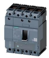
circuit breaker 3VA1 IEC frame 160 breaking capacity class N lcu=25kA @ 415V 4-pole, line protection TM220, ATFM, In=40A overload protection Ir=28A...40A short-circuit protection Ii=10 x In N conductor unprotected nut keeper kit
