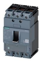
circuit breaker 3VA1 IEC frame 160 breaking capacity class N Icu=25kA @ 415V 3-pole, line protection TM220, ATFM, In=40A overload protection Ir=28A...40A short-circuit protection Ii=10 x In clamp connection
