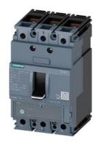
circuit breaker 3VA1 IEC frame 160 breaking capacity class N Icu=25kA @ 415V 3-pole, line protection TM220, ATFM, In=40A overload protection Ir=28A...40A short-circuit protection Ii=10 x In nut keeper kit
