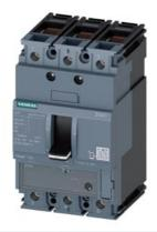
circuit breaker 3VA1 IEC frame 160 breaking capacity class M Icu=55kA @ 415V 3-pole, starter protection TM120M, AM, In=32A without overload protection short-circuit protection Ii=7...16 x In clamp connection
