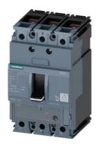
circuit breaker 3VA1 IEC frame 160 breaking capacity class M Icu=55kA @ 415V 3-pole, starter protection TM120M, AM, In=32A without overload protection short-circuit protection Ii=7...16 x In nut keeper kit
