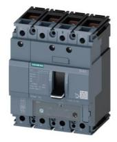
circuit breaker 3VA1 IEC frame 160 breaking capacity class M Icu=55kA @ 415V 4-pole, line protection TM240, ATAM, In=32A overload protection Ir=22A...32A short-circuit protection Ii=5...10 x In N conductor protection 100% nut keeper kit
