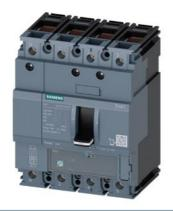
circuit breaker 3VA1 IEC frame 160 breaking capacity class M Icu=55kA @ 415V 4-pole, line protection TM220, ATFM, In=32A overload protection Ir=22A...32A short-circuit protection Ii=10 x In N conductor protection 100% clamp connection
