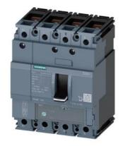
circuit breaker 3VA1 IEC frame 160 breaking capacity class M Icu=55kA @ 415V 4-pole, line protection TM220, ATFM, In=32A overload protection Ir=22A...32A short-circuit protection Ii=10 x In N conductor protection 100% nut keeper kit
