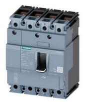
circuit breaker 3VA1 IEC frame 160 breaking capacity class S Icu=36kA @ 415V 4-pole, line protection TM210, FTFM, In=32A overload protection Ir=32A fixed short-circuit protection Ii=10 x In N conductor protection 100% nut keeper kit
