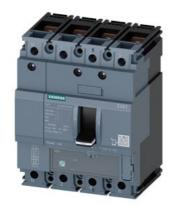
circuit breaker 3VA1 IEC frame 160 breaking capacity class S Icu=36kA @ 415V 4-pole, line protection TM220, ATFM, In=32A overload protection Ir=22A...32A short-circuit protection Ii=10 x In N conductor unprotected nut keeper kit
