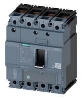
circuit breaker 3VA1 IEC frame 160 breaking capacity class S Icu=36kA @ 415V 4-pole, line protection TM220, ATFM, In=25A overload protection Ir=18A...25A short-circuit protection Ii=12.8 x In N conductor unprotected nut keeper kit
