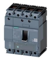
circuit breaker 3VA1 IEC frame 160 breaking capacity class N Icu=25kA @ 415V 4-pole, line protection TM220, ATFM, In=25A overload protection Ir=18A...25A short-circuit protection Ii=12.8 x In N conductor unprotected nut keeper kit
