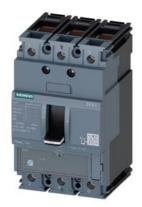
circuit breaker 3VA1 IEC frame 160 breaking capacity class N Icu=25kA @ 415V 3-pole, line protection TM220, ATFM, In=25A overload protection Ir=18A...25A short-circuit protection Ii=12.8 x In clamp connection
