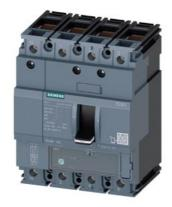
circuit breaker 3VA1 IEC frame 160 breaking capacity class M Icu=55kA @ 415V 4-pole, line protection TM220, ATFM, In=20A overload protection Ir=14A...20A short-circuit protection Ii=16 x In N conductor protection 100% clamp connection
