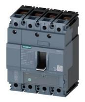
circuit breaker 3VA1 IEC frame 160 breaking capacity class M Icu=55kA @ 415V 4-pole, line protection TM220, ATFM, In=20A overload protection Ir=14A...20A short-circuit protection Ii=16 x In N conductor protection 100% nut keeper kit
