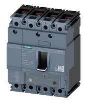
circuit breaker 3VA1 IEC frame 160 breaking capacity class M Icu=55kA @ 415V 4-pole, line protection TM240, ATAM, In=20A overload protection Ir=14A...20A short-circuit protection Ii=8...16 x In N conductor unprotected nut keeper kit
