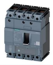
circuit breaker 3VA1 IEC frame 160 breaking capacity class M Icu=55kA @ 415V 4-pole, line protection TM220, ATFM, In=20A overload protection Ir=14A...20A short-circuit protection Ii=16 x In N conductor unprotected nut keeper kit
