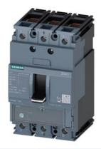
circuit breaker 3VA1 IEC frame 160 breaking capacity class M Icu=55kA @ 415V 3-pole, line protection TM220, ATFM, In=20A overload protection Ir=14A...20A short-circuit protection Ii=16 x In clamp connection
