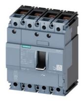
circuit breaker 3VA1 IEC frame 160 breaking capacity class N Icu=25kA @ 415V 4-pole, line protection TM210, FTFM, In=20A overload protection Ir=20A fixed short-circuit protection Ii=16 x In N conductor protection 100% nut keeper kit
