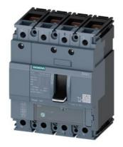
circuit breaker 3VA1 IEC frame 160 breaking capacity class S Icu=36kA @ 415V 4-pole, line protection TM220, ATFM, In=160A overload protection Ir=112A...160A short-circuit protection Ii=10 x In N conductor unprotected nut keeper kit
