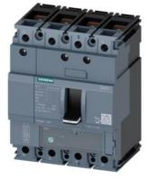
circuit breaker 3VA1 IEC frame 160 breaking capacity class N Icu=25kA @ 415V 4-pole, line protection TM220, ATFM, In=160A overload protection Ir=112A...160A short-circuit protection Ii=10 x In N conductor unprotected nut keeper kit
