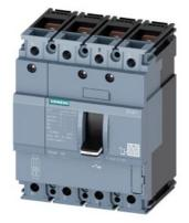
circuit breaker 3VA1 IEC frame 160 breaking capacity class M Icu=55kA @ 415V 4-pole, line protection TM210, FTFM, In=125A overload protection Ir=125A fixed short-circuit protection Ii=10 x In N conductor protection 50% nut keeper kit
